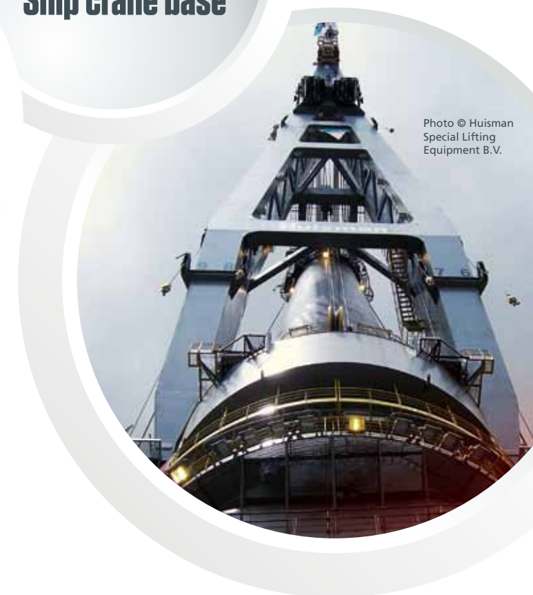
Pedestal for a 5000-t Ship crane base
